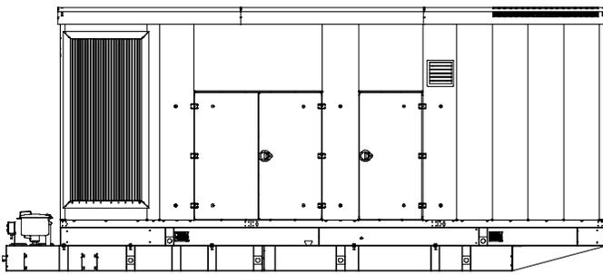
Level 2 Sound Enclosure with Subbase Fuel Tank
