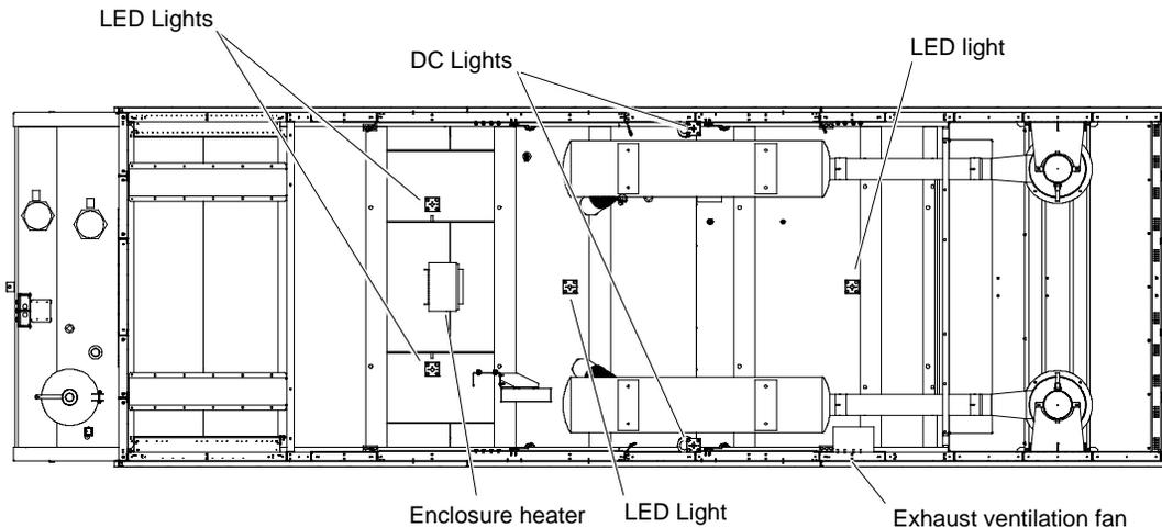
Side view of SL2 enclosure, shown with side panels removed for illustration only:
